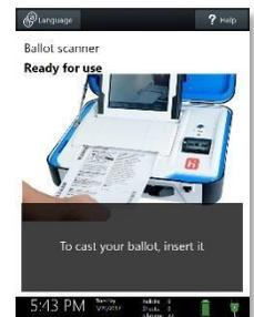
2. The voter removes the ballot privacy sleeve (if applicable) and inserts the voted ballot into Verity Scan. Flashing green arrows indicate the location and direction of the scanner feed. Ballots must be fed short-edge first, but may otherwise be scanned in any orientation. ▶
