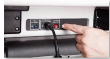
**NOTE:** The Verity power cord has a locking connector. When inserting the connector into a Verity device, it will make a small "click." To disconnect the power cord, grasp the cord at the base of the black connector molding where it connects to the Verity device, and slide back the sleeve. This will unlock the connection so that the cord may be removed.
