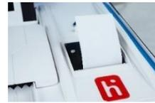
2. To open the paper compartment: While standing in front of the device, pull the lever on the top of the printer cover towards you, and then lift up to open the paper compartment. ▶
