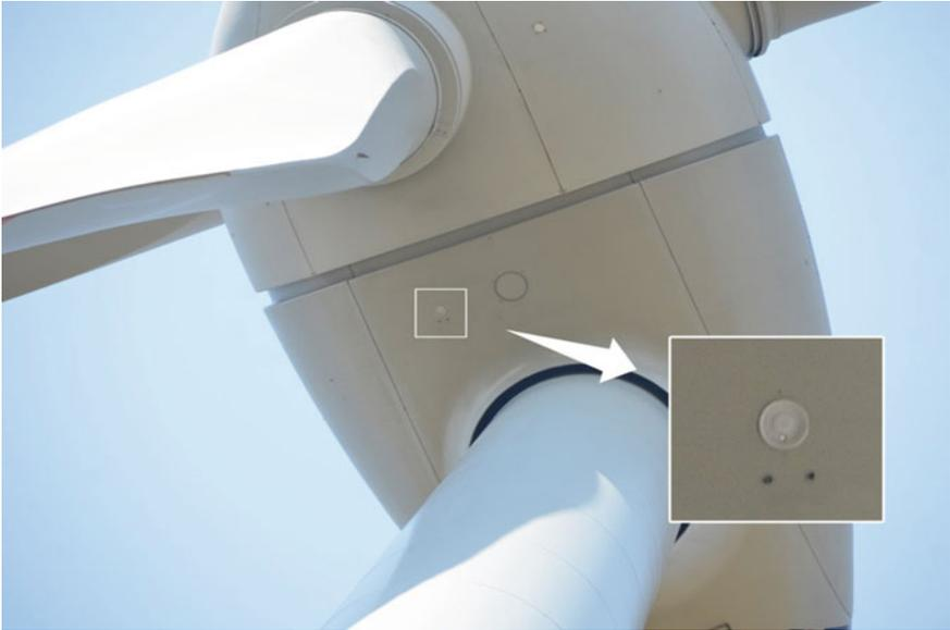
**Fig. 2** Microphone mounted in a disc in the *bottom* of a nacelle (highlighted area on the *left*). The inlay on the *right* shows this area at a larger scale. The microphone disc has a *light grey* colour and the two *dark spots below* it are additional sensors (e.g. temperature) (Color figure online)
